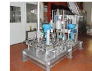
Prototype of hydrogen separation membrane unit
