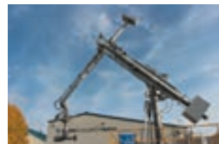
Marine loading arm for liquefied hydrogen
