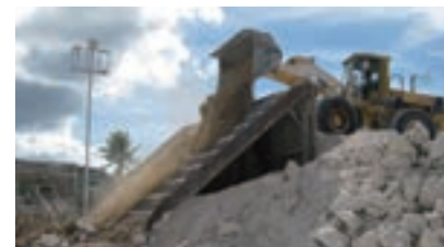
Primary screening of mineral phosphate produced in Nauru after mining
