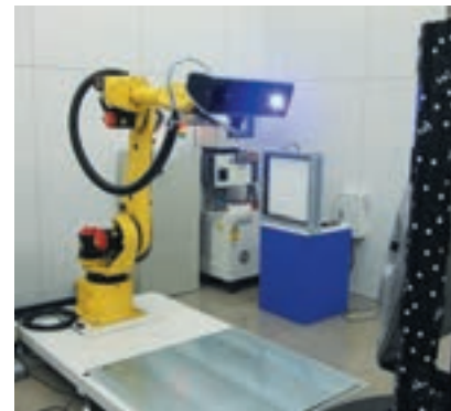
Automatic measurement equipment that uses a robotic arm
