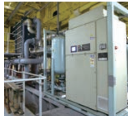
Hydrocurrent™ Organic Rankine Cycle (ORC) 125 EJW shipboard heat recovery system
