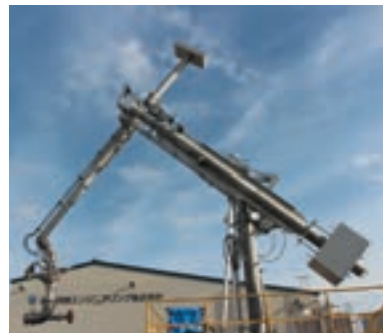
Marine loading arm for liquefied hydrogen
