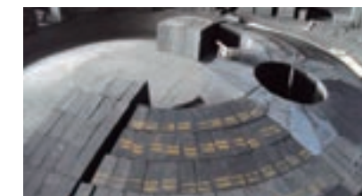
Checking magnesium-carbonate bricks in the form of temporary assembly before shipping-out
