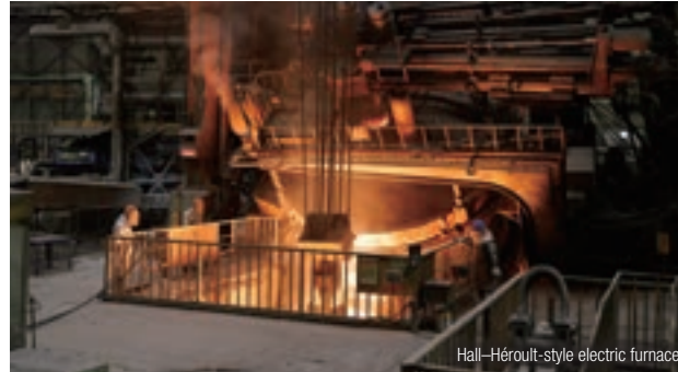
Hall-Héroult-style electric furnace
