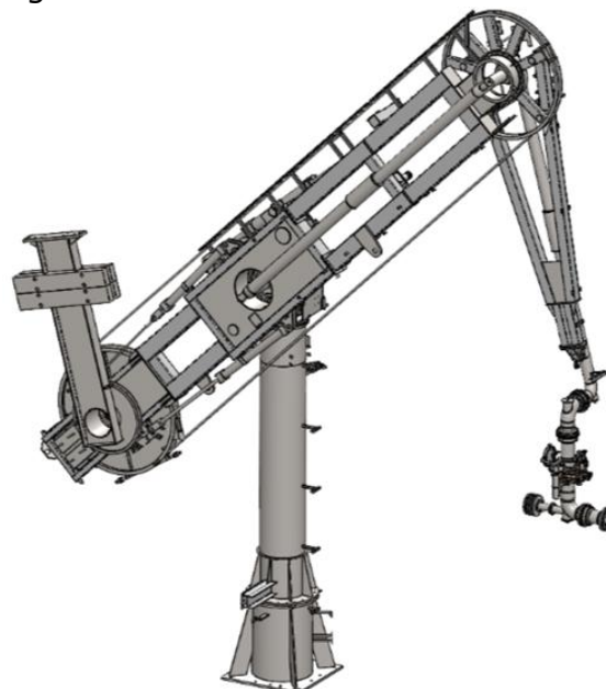
Figure 1: Image of Liquefied Hydrogen Loading Arm
