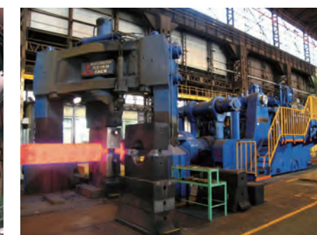
2,000 ton hydraulic forging press
