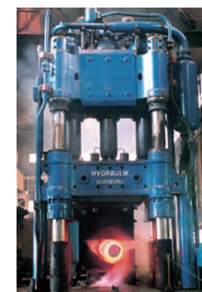
6,000 ton water-pressured forging press
